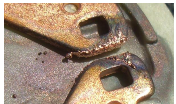
Figure 9 Degraded Gaps of a Station Class Arrester
